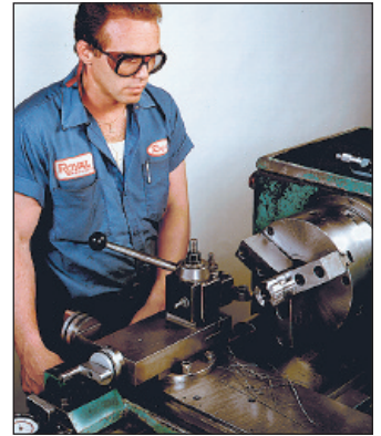
Royal strives for next-day delivery on all collet chuck orders. Here, a drawtube adapter is machined from a partially-finished blank to reduce lead time.
