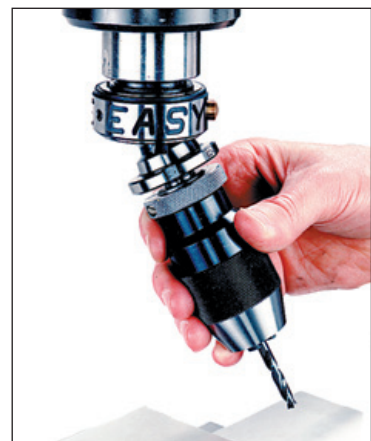
2. Loading drill chuck holder and drill into body.
