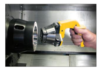
3. In its compressed state, the collet can then be inserted into the collet chuck, where the hooks on the rear of the collet segments become axially aligned with a retaining groove in the chuck.
