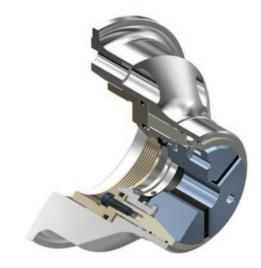
4. Releasing the installation tool allows the collet to spring open, seating the hooks in the groove and drawing the matching ID/OD tapers into full, positive contact. The collet is now installed.
