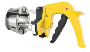
The installation tool incorporates steel pins that align with reamed holes on the collet face. When these pins engage the face holes and the trigger on the tool is actuated, the collet becomes temporarily compressed.
